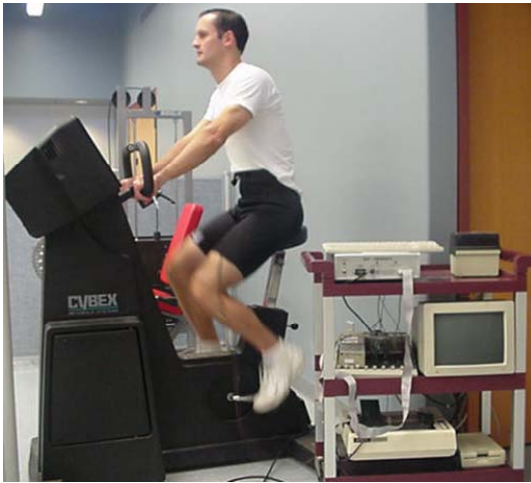
Figure 7. Experimental setup for the skin temperature measurement during stationary cycling.
