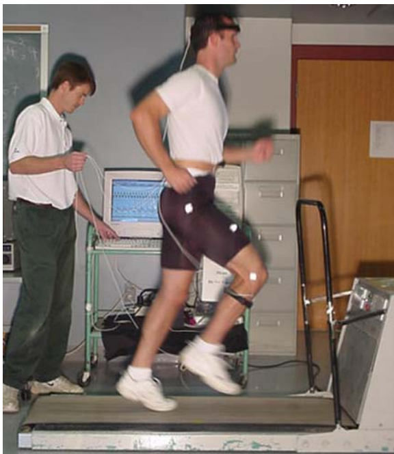
Figure 6. Experimental setup for the head and tibial shock attenuation measurement.
