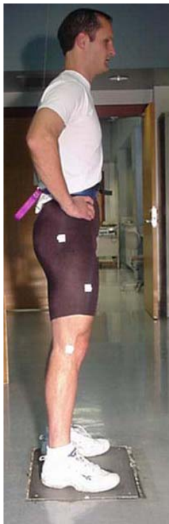
Figure 2. Experimental setup for measurement of muscle oscillation. Reflective markers are shown attached to the hip, knee and mid-thigh.
